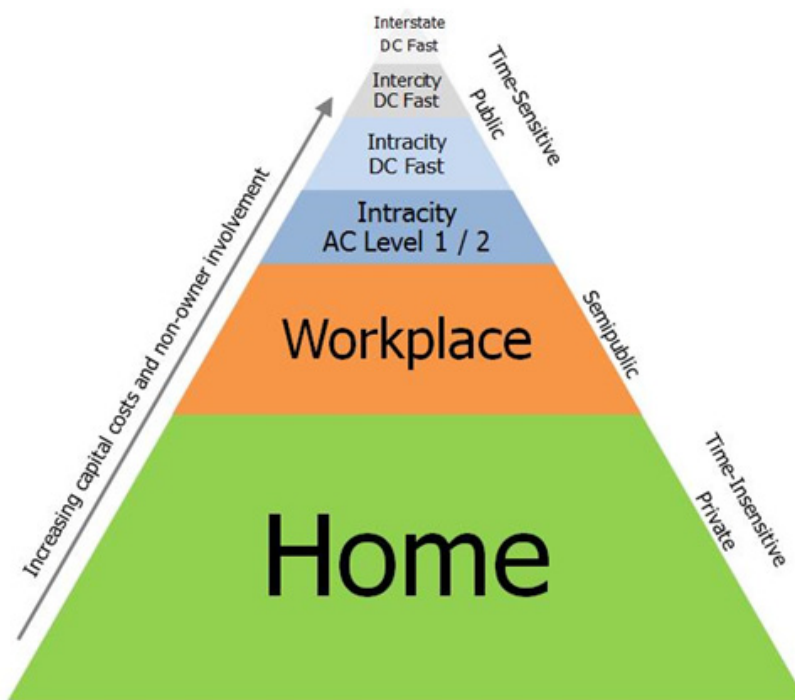
FIGURE 5-1 PEV charging infrastructure categories, ranked by their likely importance to PEV deployment, with the most important, home charging, on the bottom, and the least important, interstate DC fast charging, at the top. NOTE: AC, alternating current; DC, direct current.
